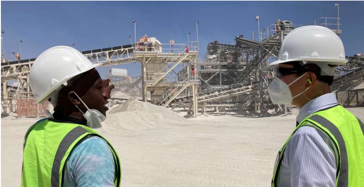
Ambassador Nishimaki (right) being shown the start of the processing plant, by Muta Shiwedha the tin and tantalum plant supervisor, consisting of a four-stage crushing circuit followed by a three-stage concentrating circuit. The concentrating circuit includes dense medium separation (DMS), fine gravity concentration and wet high-intensity magnetic separation (WHIMS) modules.
