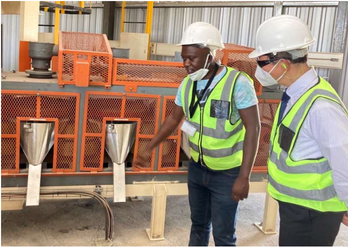
Ambassador Nishimaki (right) taking a closer look at the wet high-intensity magnetic separation (WHIMS) modules for the production of salable tin and tantalum concentrates.
